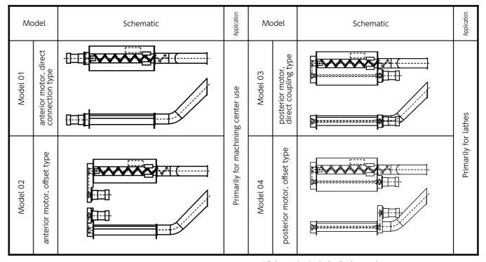
\* Schematics include discharge ducts.
